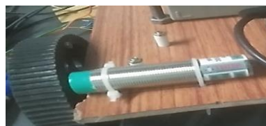
Figure.9. Inductive proximity sensor
